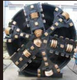
Tunneling machine cutter head
